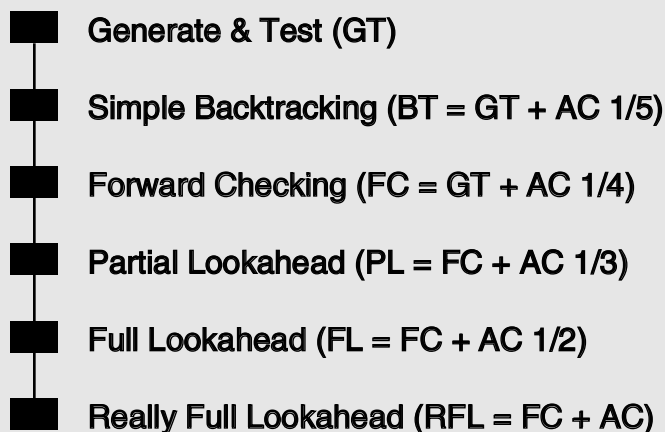
Figure 6. Different Constraint-Satisfaction Algorithms Depicted as a Combination of Tree Searching and Different Degrees of Constraint Propagation.
